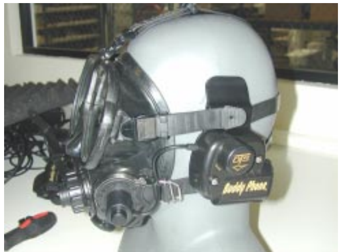
A fully installed ScubaPro Buddy Phone®
