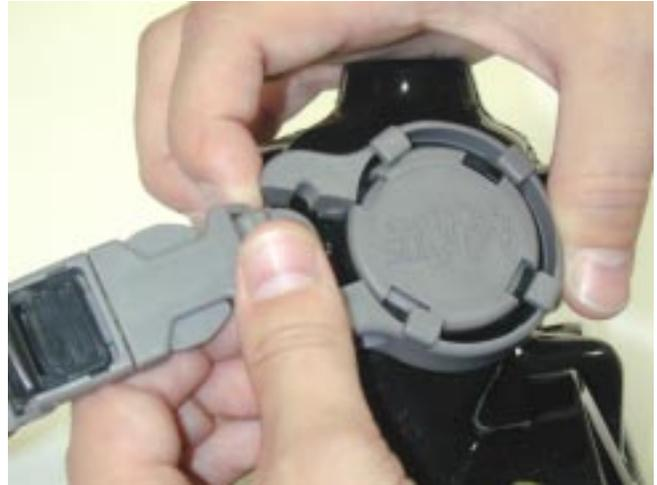
2. Open the clamp that attaches the mask strap, releasing the tabs that hold the cap onto the accessory port. Remove the cap from the port.
