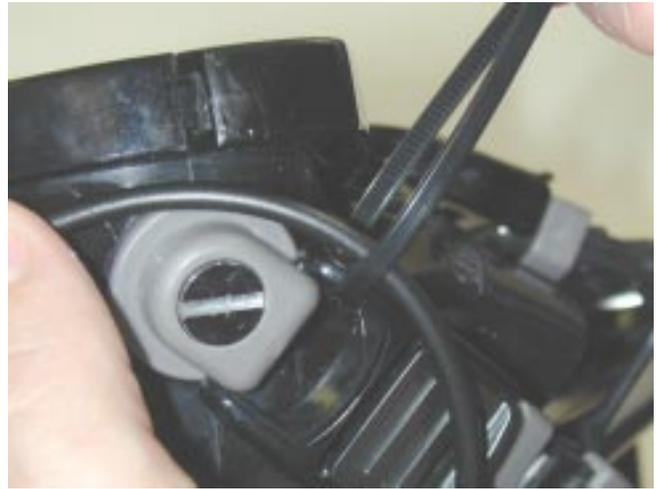
7. Install a tie wrap to secure loosely the Buddy Phone® cable to the upper prong of the upper left mask strap buckle (where the buckle attaches to the buckle holder on the mask). Cut off any extra length of tie wrap.
