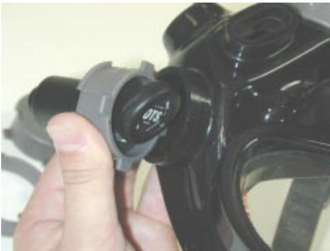
3. Insert the microphone/push-to-talk (PTT) module of the Buddy Phone® fully into the open accessory port so that the module rests evenly along the opening. Match the orientation of the opposite port's cap. The microphone should be positioned at a 45-degree angle relative to the front inner surface of the mask.
