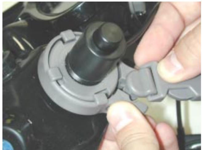
4. Install the clamp onto the PTT assembly cap, ensuring the strap buckle is attached to the clamp. Close the clamp's tabs onto the cap so that the assembly is fastened securely.
