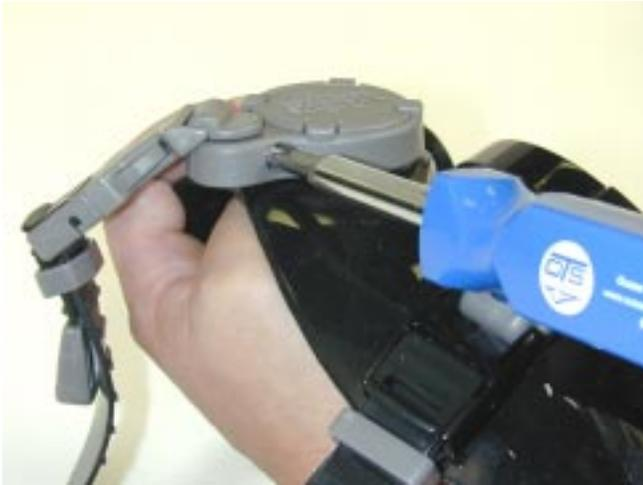
1. Remove the screw that secures the clamp on the diver's left accessory port of the mask. Set the screw and nut aside.
